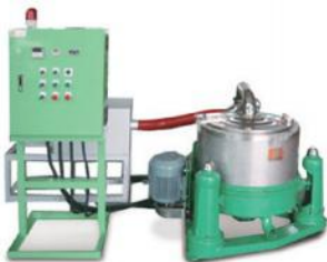
HE-26 centrifugal dryer with hot air blower
