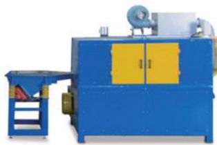
Drum dryer with hot air
