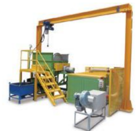
Rotary barrel dryer with hot air
