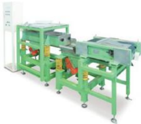
Vibratory separator with magnetic
