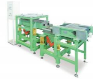
Vibratory separator with magnetic
