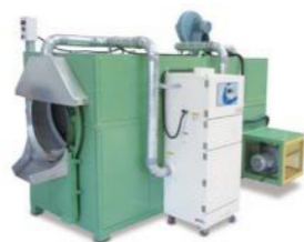
Drum dryer using corncob
