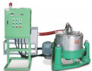
HE-26 centrifugal dryer with hot air blower
